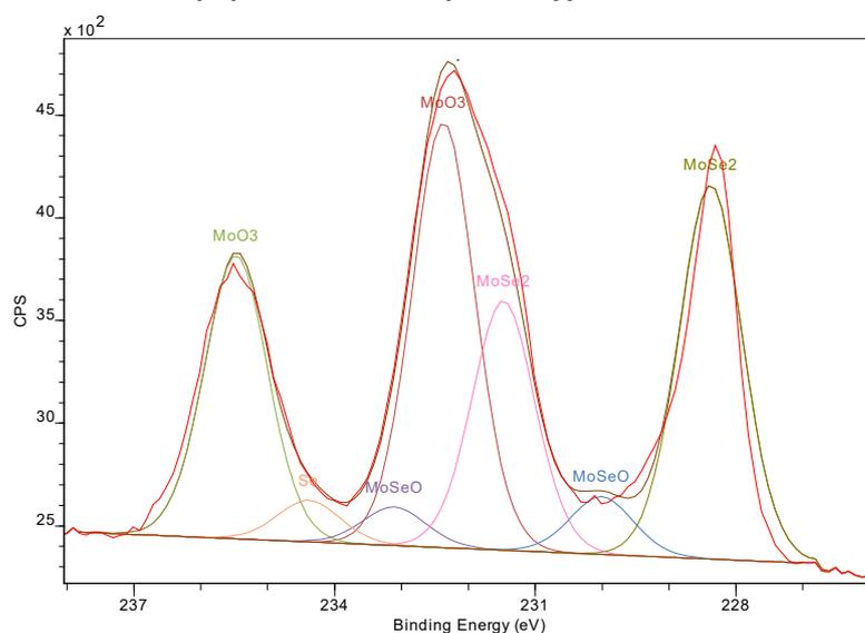
Figure 2: XPS data indicating the formation of MoSe<sub>2</sub> via AACVD but also demonstrating the presence of significant amounts of oxides.
