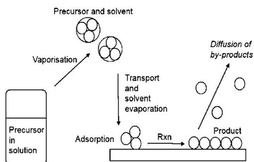
Figure 1: Schematic of the aerosol assisted chemical vapour deposition process.<sup>2</sup>
