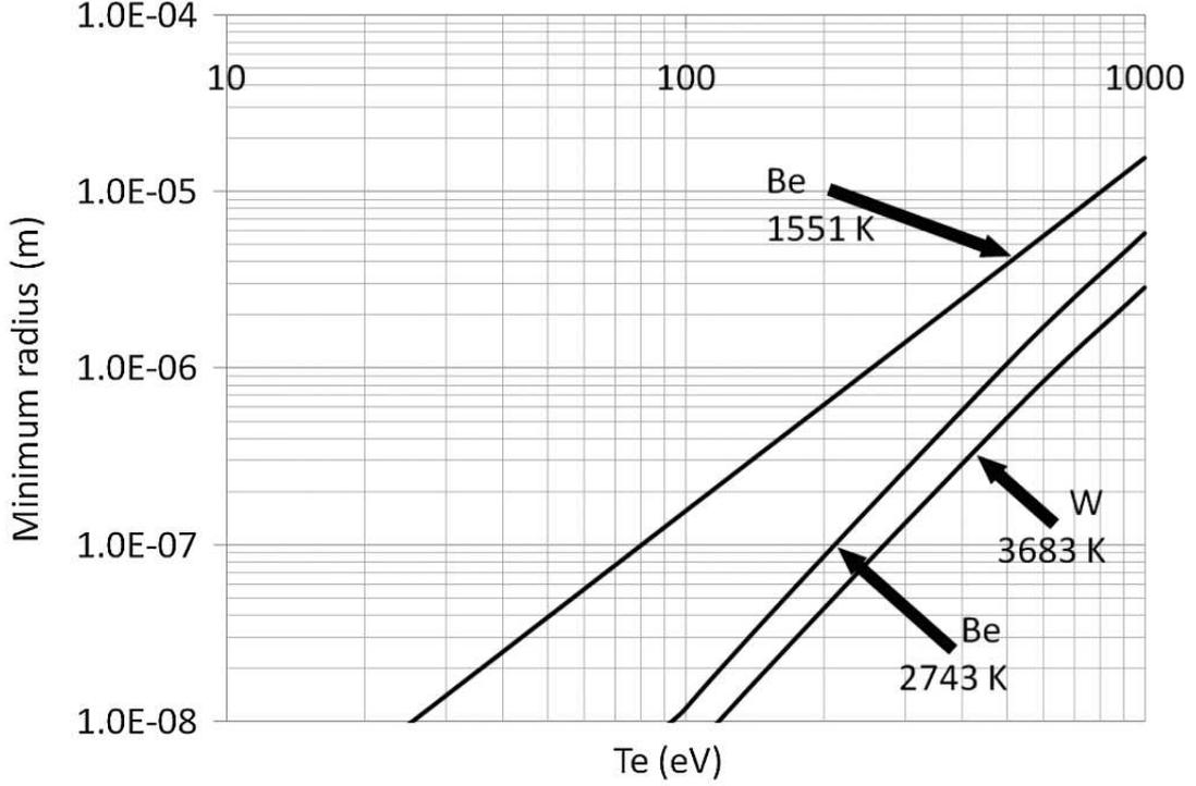
**Figure 1:** The minimum stable radius of beryllium and tungsten droplets in a fusion plasma as a function of electron temperature in energy units; for conversion to Kelvin  $1 \text{ eV} = 11600 \text{ K}$ . Reproduced from [4].
