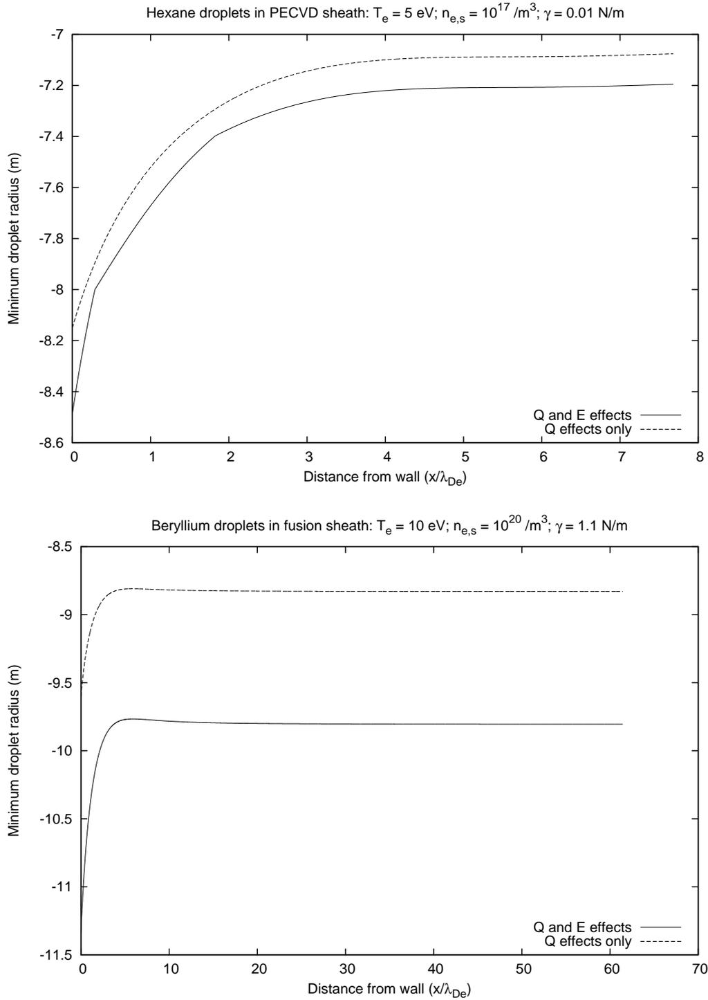
**Figure 2:** The minimum stable droplet radius for droplets in typical PECVD and fusion plasma sheaths. Droplet stability improves when electric field effects are considered, and droplets close to the wall are shown to be more stable.
