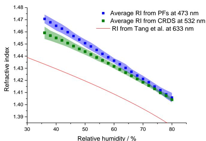
*Figure 1: The average RI of 5 ammonium bisulfate droplets (indicated by the blue and green squares which correspond to 473 nm and 532 nm respectively), the shaded area corresponds to the standard deviation in RI, measurements at 633 nm by Tang et al.<sup>3,4</sup> are shown in red.*
